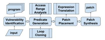
Fig. 1: Workflow of Senx: each rounded rectangle represents a step in Senx's patch generation, each rectangle with vertical bars represents a component of Senx.
