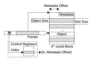
Figure 7: Subheap Scheme. The dashed box represents an implementation defined function that maps assigned tag bits to memory block size and metadata offset.
