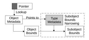
Figure 1: Pointer Bounds Retrieval in Previous Taggedpointer Schemes using Object Metadata. The subobject bounds narrowing is unique to EffectiveSan [14].
