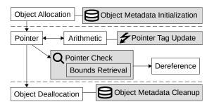
Figure 3: Operations Instrumented by In-Fat Pointer. In-Fat Pointer introduce new instructions for hardware-assisted pointer checks, bounds retrieval (promote), and pointer tag updates.
