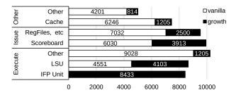
Figure 13: LUT Increase in the Modified Processor
